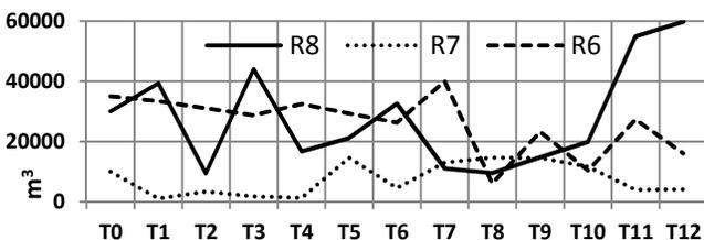
Fig. 9. Storage in 3 reservoirs. T0 is the initial state. Odd labels are for peak periods, even labels are off-peak periods.
