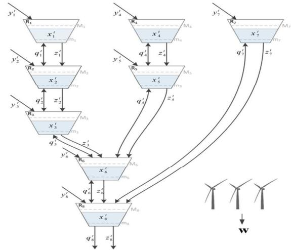
Fig. 7. Scheme for the wind-hydro test power system with a cascading arrangement of reservoirs, different in capacity, constraints and inflows.
